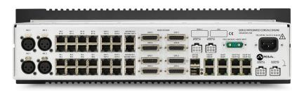
Let's take a look around back, shall we? You'll find everything you need for an average, medium-sized studio: 4 mic inputs with selectable Phantom power, 16 stereo analog inputs and 8 stereo analog outputs, 2 AES/EBU inputs and 2 AES/EBU outputs, 8 GPIO machine-control logic ports (each with 5 opto-isolated inputs and 5 outputs).
